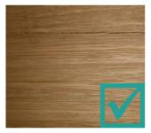
Checking is acceptable provided individual length does not exceed 250mm and width does not exceed 1mm.
