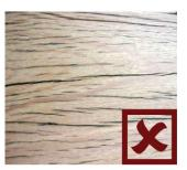
Checking is acceptable provided individual length does not exceed 250mm and width does not exceed 2mm.
