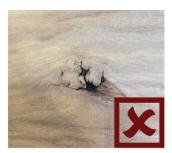
Gum Veins of less than 250mm in length and 2mm in width are acceptable.
