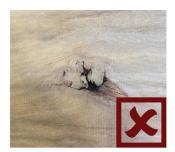
Gum Veins of less than 250mm in length and 2mm in width are acceptable.
